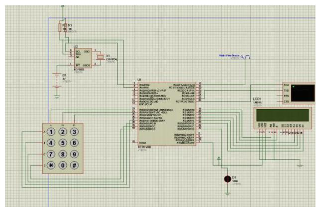
Fig. 5. Schematic Diagram of Prepaid Smart Water Meter
