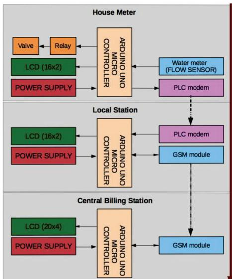
Fig. 7. System Block Diagram
